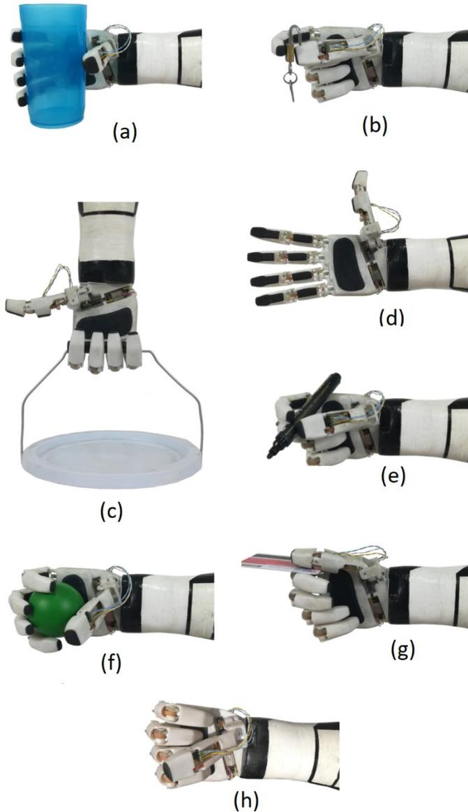
Fig. 1. Types of grasp implemented on the robotic hand: (a) Cylindrical grasp, (b) Tip grasp, (c) Hook grasp, (d) Open hand, (e) Palmar grasp, (f) Spherical grasp, (g) Lateral grasp, (h) Fist.
