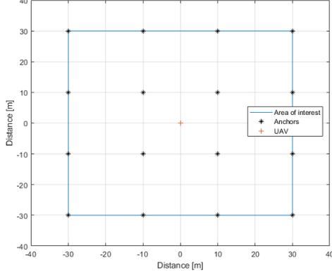
Fig. 2. Simulation scenario where a UAV flies randomly in an area of  $30 \times 30$  m with a square grid array of anchors.
