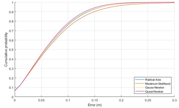
Fig. 7. CDF of the estimation error obtained for each positioning algorithm.
