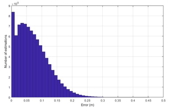
Fig. 5. Histogram of the estimation error for the Gauss-Newton algorithm.
