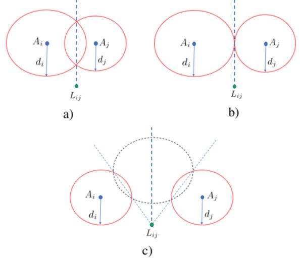
Fig. 1. Radical axis cases of two circles: a) when both circles touch in two points, b) when both circles touch in one point and c) when both circles do not touch each other
