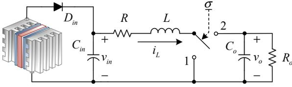
Fig. 1. Fuel-cell system composed by a hydrogen fuel-cell stack, a boost cd-cd converter and a resistive load. Rated output power  $P_o = 853.33$  W.
