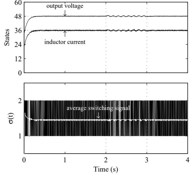
Fig. 2. Fuel-cell system response using switching rule  $\sigma(t)$  in (9) at nominal output power  $P_o = 853.33$  W. The desired equilibrium point is computed as  $x_e = [35.92, 48.00]^\top$  with  $E_{in} = 24$  V and nominal load  $R_o = 2.7 \Omega$ . A disturbance  $w(t) = \sin(16\pi t)$  appears at time  $t \in [2, 3]$ . Data is down-sampled for clarity of display.
