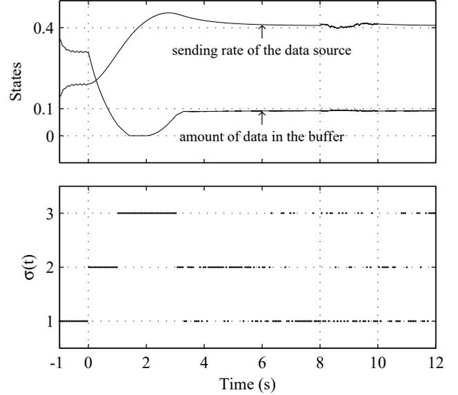
Fig. 3. Congestion control of a communication network using switching rule  $\sigma(t)$  in (9). The desired amount of data in the buffer is set to  $y_d = 0.2$ . High frequency measurement noise  $w(t)$  appears at time  $t \in [8, 10]$ . The top panel shows the states of the system. The bottom panel depicts the switching signal  $\sigma$ . Data is down-sampled for clarity of display.
