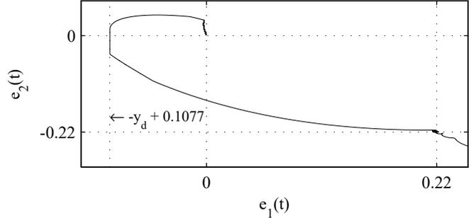
Fig. 4. Error trajectories of system (21)-(22) decaying exponentially fast towards the origin as ensured by Theorem 1.
