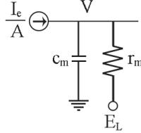
Fig 2. RC circuit equivalent to the neuron membrane. Based on [10]
