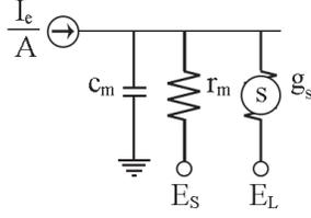
Fig 4. Equivalent RC circuit with synaptic conductance. Base on [10]
