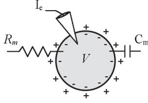
Fig 1. Analogous representation of a neuron cell. Based on [10]
