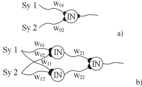
Fig 9. Feedforward neural architecture. a)Architecture “A”, b)Architecture “B”
