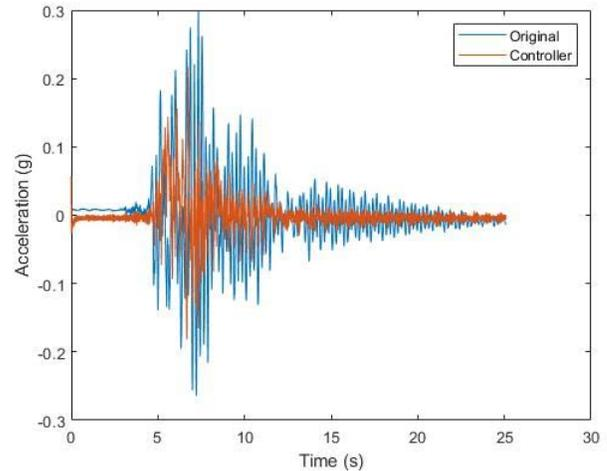
Fig. 7. Acceleration response from substructure 2: uncontrolled (blue trace) and controlled (orange trace) using the model reference controller.
