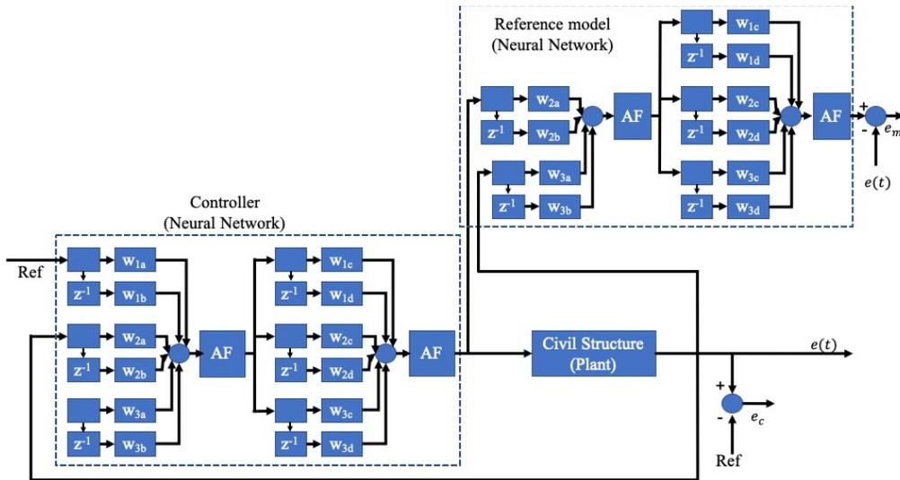
Fig. 2. Detailed Reference Neural Controller Block Diagram.
