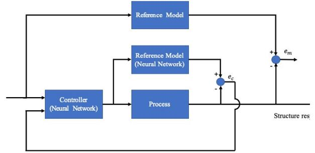
Fig. 1. Model Reference Neural Controller Block Diagram.
