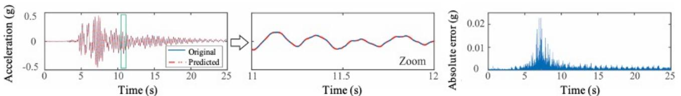
Fig. 6. Predicted response of floor 2 using the NN model
