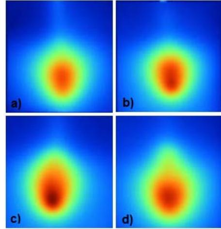
Figure 2. Thermal images obtained with a thermographic camera Fluke Ti32. a) MTM antenna, b) MTM-C antenna, c) DS antenna and d) DS-C antenna.
