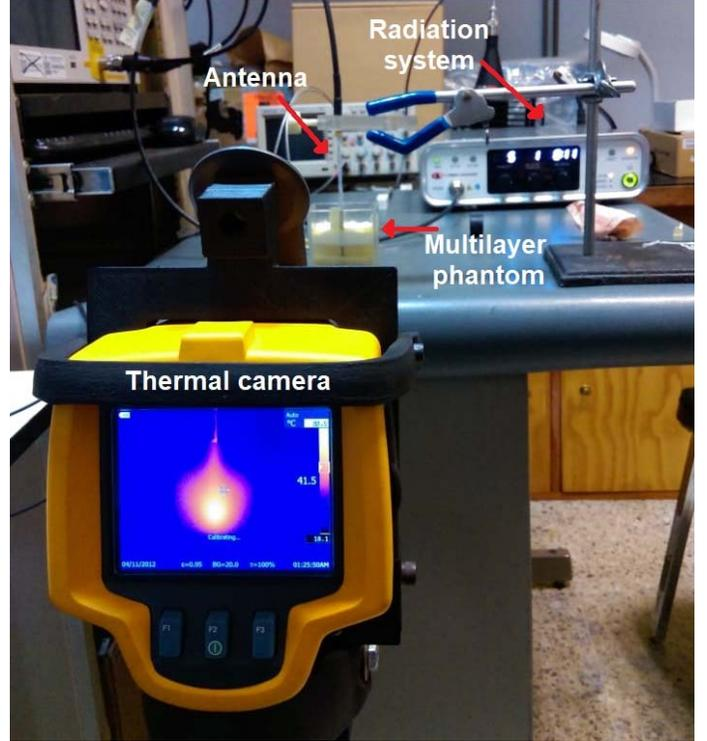
Figure 1. Experimental configuration to obtain the thermal images in microwave ablations by using interstitial antennas.
