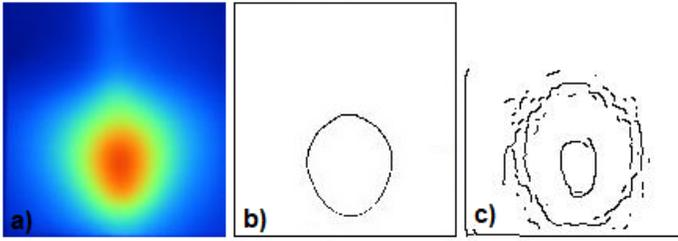
Figure 4. Contour of the temperature distribution of an MTM antenna. a) thermal image, b) proposed algorithm and c) edge detection using Canny method.
