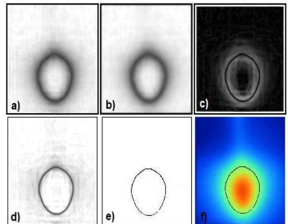
Figure 3. Processing of the thermal image of an MTM antenna. a) channel  $I$  of the thermal image, b) channel  $I$  filtered with the Gaussian filter, c) intensity gradient, d) result of the sum between image 3b and 3c, e) black and white mask and f) positioning of the mask on the original thermal image.
