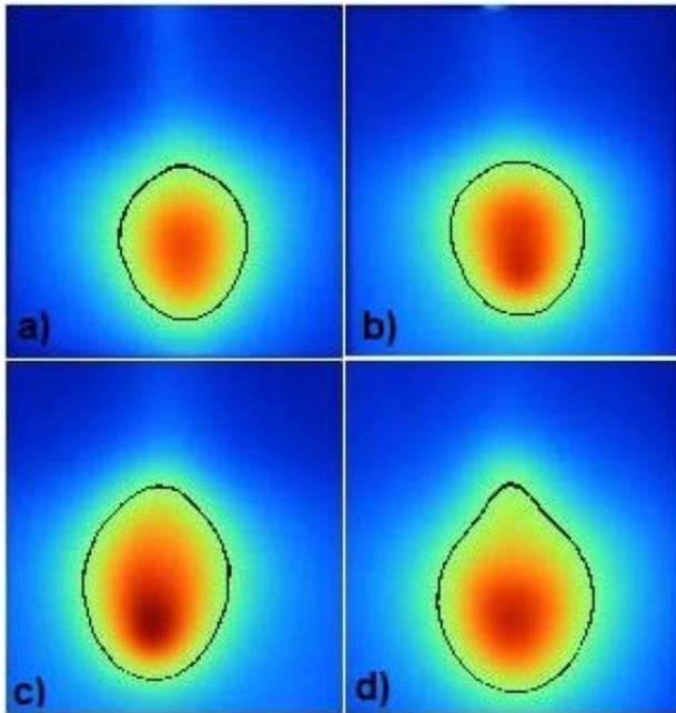
Figure 6. Contour of the temperature distribution generated by micro-coaxial antennas. a) MTM antenna, b) MTM-C antenna, c) DS antenna and d) DS-C antenna.
