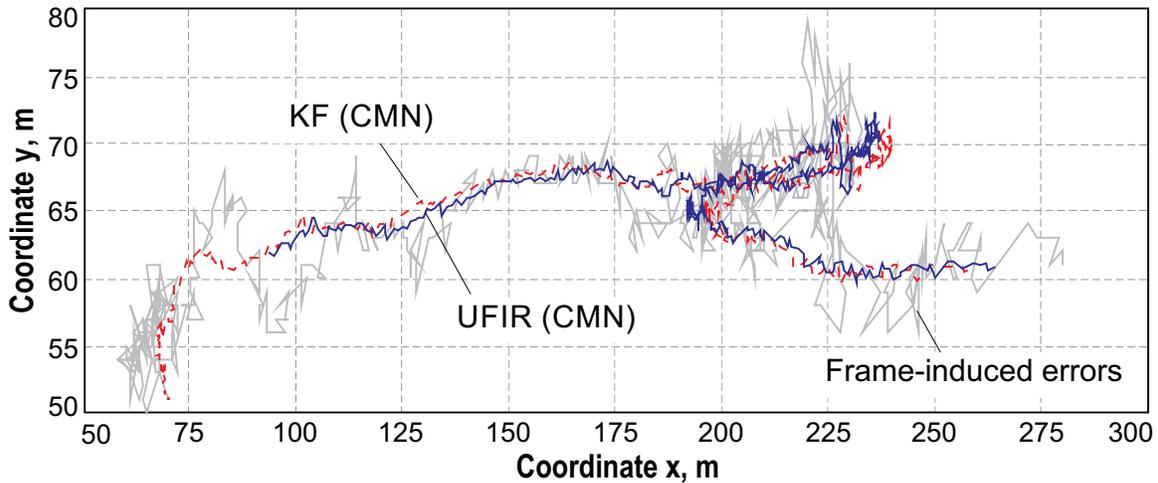
Fig. 4. Suppressing the frame slow variations associated with CMN and fast variations associated with white noise in x-y plane of the “Car4” benchmark using modified KF and UFIR filter.
