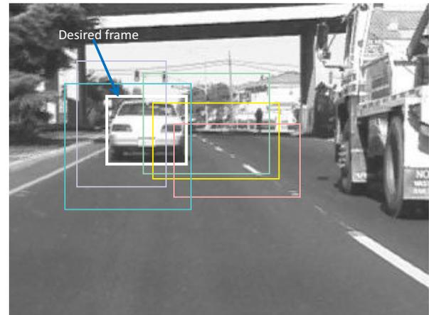
Fig. 1. Possible appearances of the video camera image frame in visual object tracking due to the object dynamics and low frame rate. A desirable frame is white.
