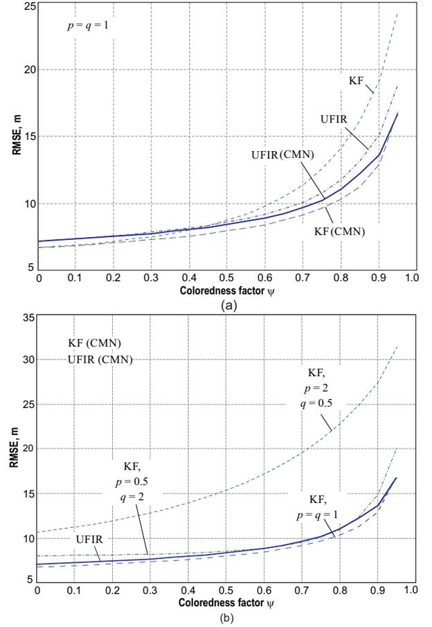
Fig. 2. Typical RMSEs produced by the modified KF and UFIR filter ( $N_{\text{opt}} = 20$ ) as functions of the coloredness factor  $\psi$  for the two-state tracking model under: (a) ideal conditions,  $p = q = 1$ , and (b) errors in the noise statistics,  $p \neq 1$  and  $q \neq 1$ .
