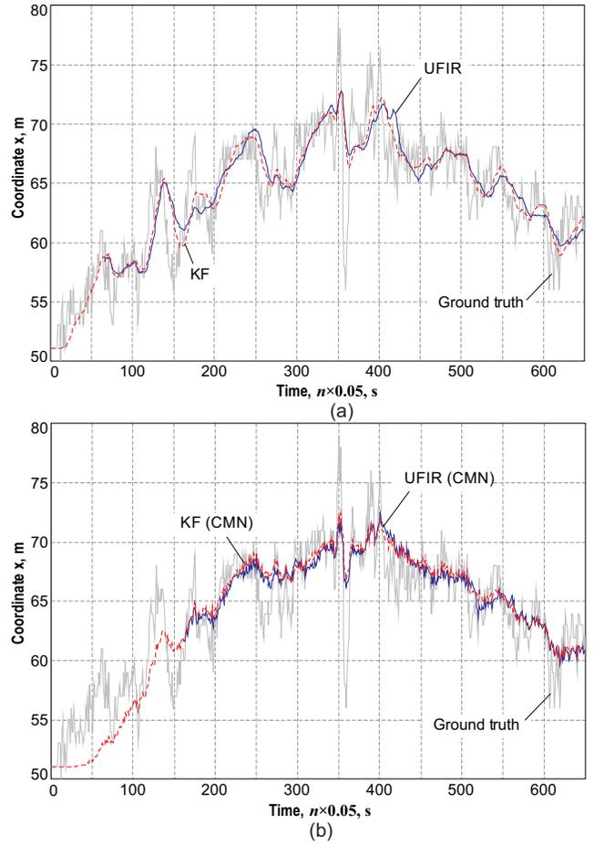
Fig. 3. A benchmark trajectory of a moving car (“Car4”) along coordinate  $x$  and its estimation using: (a) standard KF and UFIR filter ( $N = 65$ ) and (b) modified KF and UFIR filter with  $N = 160$ .
